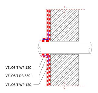
sleeve with a diameter approx. 6 mm (%") smaller than the pipe. The sleeve is made from a 12 cm (5") piece of VELOSIT DB 830. Brush plenty of VELOSIT WP 120 or 121 onto the pipe and the surrounding area. Pull the sleeve over the pipe push it with a trowel into the material. Work away from the pipe and take care not to entrap air or create wrinkles.
