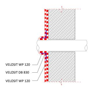
sleeve with a diameter approx. ½" (6mm) smaller than the pipe. The sleeve is made from a 5" (12 cm) piece of VELOSIT DB 830. Brush plenty of VELOSIT WP 120 or 121 onto the pipe and the surrounding area. Pull the sleeve over the pipe push it with a trowel into the material. Work away from the pipe and take care not to entrap air or create wrinkles.
