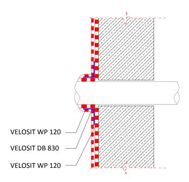
piece of VELOSIT DB 830. Brush plenty of VELOSIT WP 120 onto the pipe and the surrounding area. Pull the sleeve over the pipe push it with a trowel into the material. Work away from the pipe and take care not to entrap air or create wrinkles.
